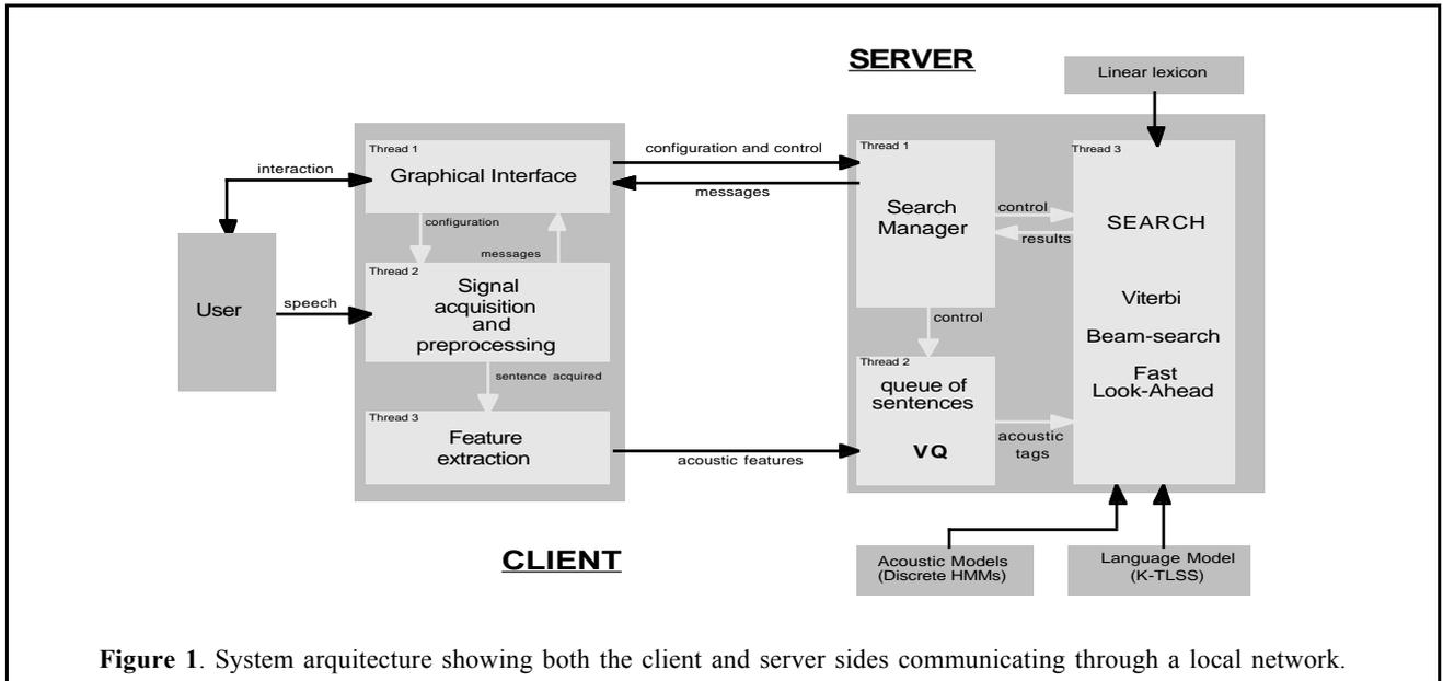
Figure 1. System architecture showing both the client and server sides communicating through a local network.
